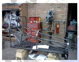
October: The front part of the chassis has been welded together. The front axle has been cut. Caitlin had worked on the wheel parts. Alex is grinded down the sides of the base frame. The round tubing was cut. Dimensions on the round tubing were being dimensioned at the same time. The floor was tack
